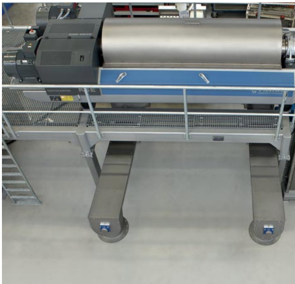
Solids discharge heavy phase (on the left), light phase (on the right)
