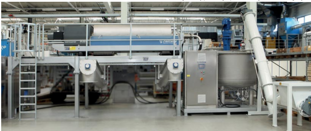
FLOTTWEG SORTICANTER® system From the left: SORTICANTER® with solids discharge, heavy phase, light phase, mixing tank and dosage system
