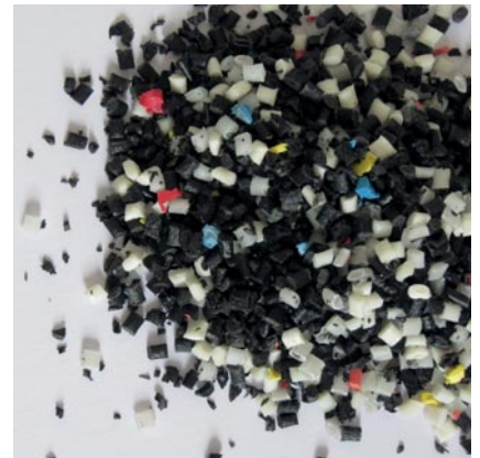
Granulate of different plastics before separation
